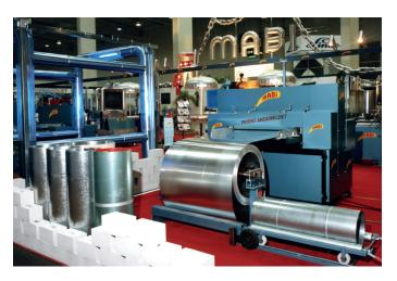
Another MABI invention: in 1994, the first MABI Bingo was delivered and unveiled at the Euroblech exhibition in Hannover. For the first time, curvatures, forms and straight pipe lengths could be produced by a single machine.
