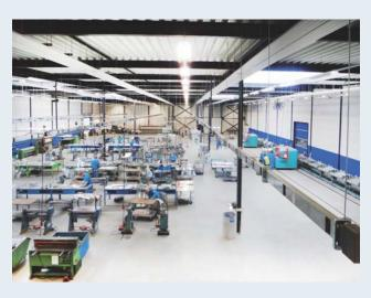
Man and machine: On the right, the double MABI line for two x eight pipe metres per minute, on the left, the team of specialists that process these pipes extremely efficiently into assembly-ready project packages.
