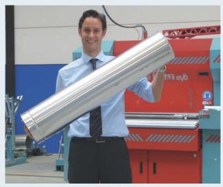
Mabi managing director Markus Biland, with the 16 4Z-EVO in the background, also known as the "Rohrblitz". This machine is completely designed for mass and individual production of insulation pipes and blanks. Straightening, cutting, punching, beading and rounding all take place consecutively in a fully automated working process. All commercial material dimensions and types - including Inox - can be processed. Including the increasingly popular sheet width 1250 mm.
