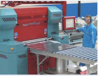
Bilfinger uses the patented top Mabi model, Bingo 2 EVO, a fully automated jack of all trades for insulation sheets, to cut shaped pieces: Double cutting system, automatic width adjustment, product coding with fast-drying ink, optimisation of sheet nesting and online programming. The machine can be fully programmed during work preparation. The coding texts can also be adapted or expanded here.
